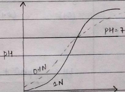
→ After addm of 100ml 1N NaOH. The pH will sharply change to 7
